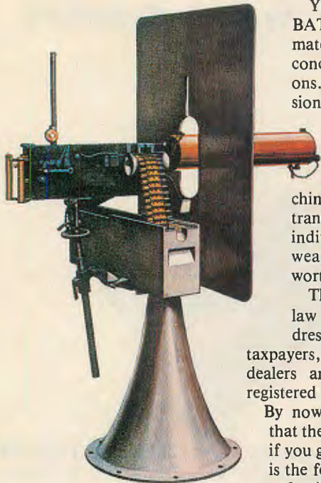
.303 Maxim on cone mounting with shield. This was a favorite naval weapon in the days of the ironclads. It was intended to keep the enemy's decks cleared and repel boarders if necessary.
